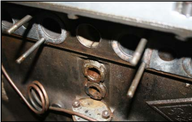
RH (driver's) side of block, after removal of inlet manifold. On this car, the flanged ends on this side are notched for a socket.
