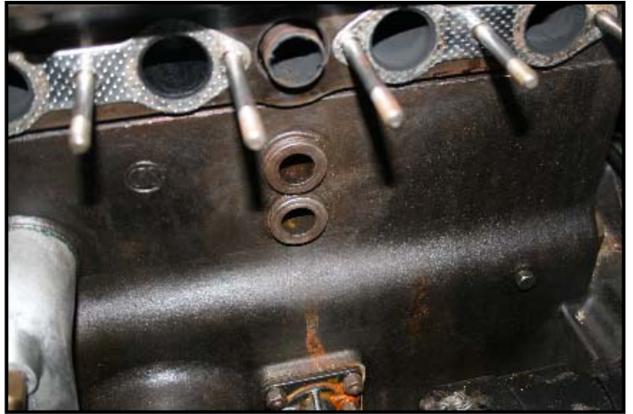
LH side, after removal of exhaust manifold, showing hot spot tube ends - flanged, on this car, with plain threaded washers.
