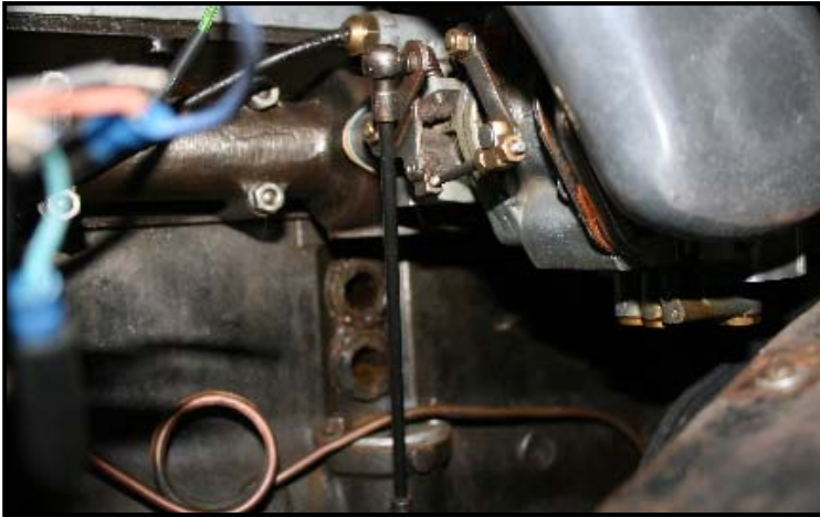
RH (driver's) side of block, looking under carburettor to ends of hot spot tubes, after removal of cast alloy elbow from manifold.
