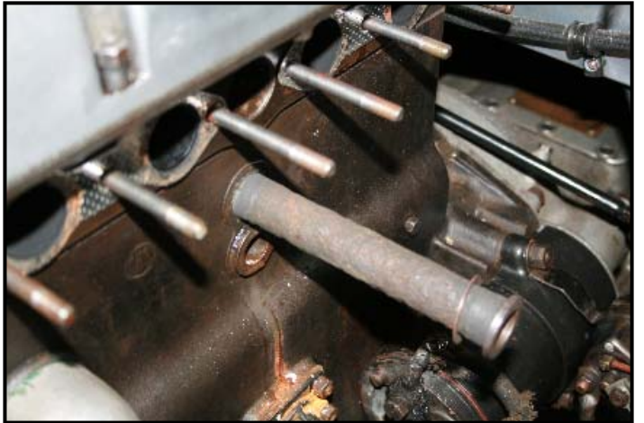
LH side of block, showing the upper of the two lower hot spot tubes being withdrawn, still with threaded and copper washers.
